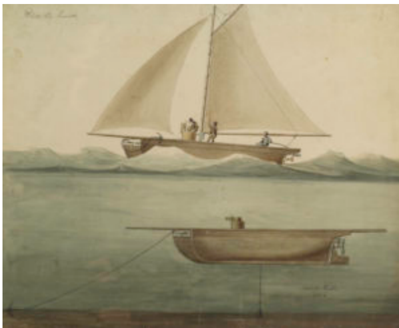
Fig. 8. Robert Fulton, Two views of Fulton's submarine, under sail and submerged. Scale one quarter of an inch to a foot., 1806. Watercolor. Manuscripts and Archives Division, The New York Public Library, Astor, Lenox and Tilden Foundations.
