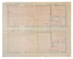
Fig. 1. Maria Chabot, two floor plans for Georgia O'Keeffe's studio with specs for radiant heating system, 1947. Graphite and colored pencil on graph paper, approximately 18 x 24 in. Verso shows a full plan for the house, including electric, gas, and water utilities. Georgia O'Keeffe Papers (MS.33), House Files, oversize box 2. Georgia O'Keeffe Museum, Michael S. Engl Family Foundation Library and Archive; photograph by the author with permission of the Georgia O'Keeffe Museum
